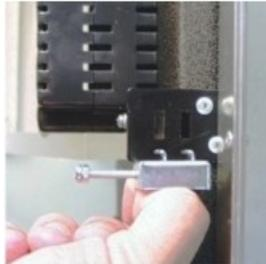
2. Tighten the screw against the enclosure surface. **Note:** Tighten DIN Clips to a maximum of 1.5 inchpounds to provide a proper seal.
