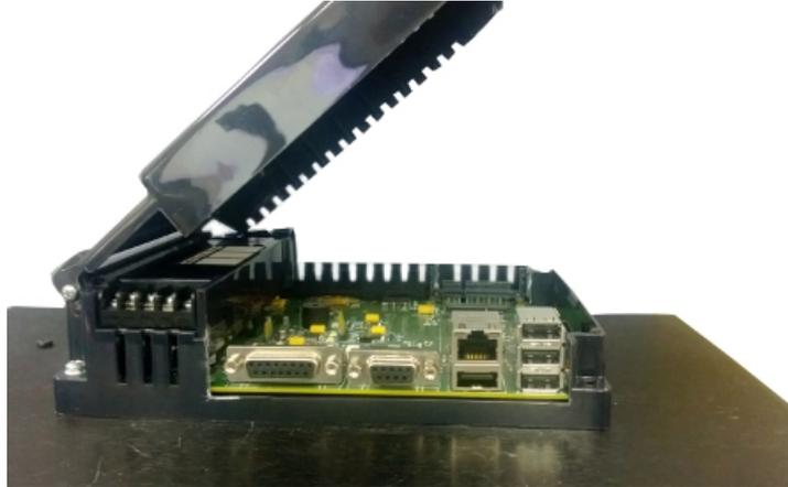
2. The battery is located in the upper-left hand corner as shown in the figure below. Remove the old battery and replace with a new 1/2 AA, 3.6 V Lithium Battery (Part Number: **UT-B**).
