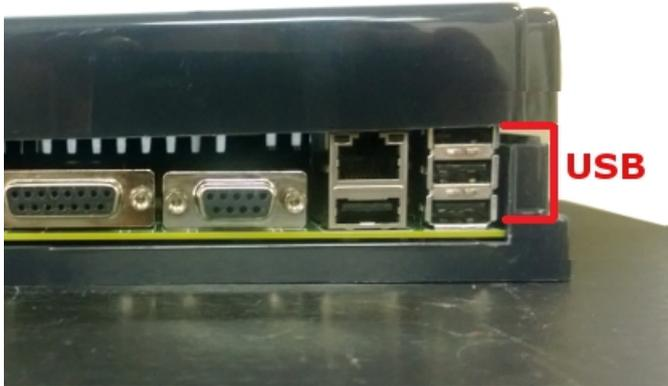
Tough Panel Plus HMIs come equipped with four USB ports. Currently the USB ports for the Tough Panel Plus are only used for USB Flash drives (data collection or program upload), and only one drive can be used at a time.
